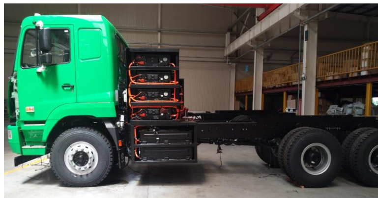
Battery Mounted on Both Sides
