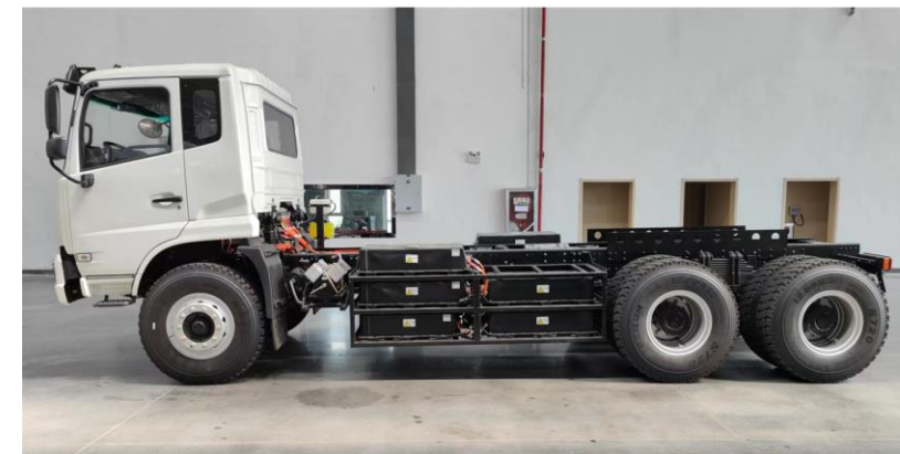
Battery Mounted on Back of the Cab
